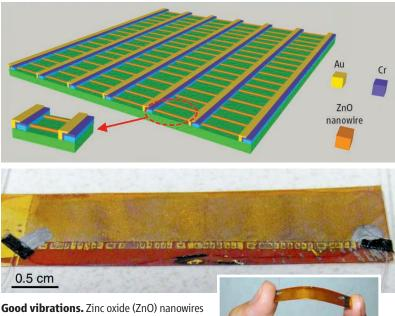
**Good vibrations.** Zinc oxide (ZnO) nanowires are grown between chromium (Cr) and gold (Au) electrodes (*top*) to make a nanogenerator that produces a high voltage when flexed.
